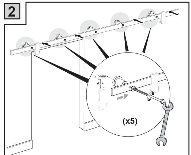
Attach the rail to the wall brackets using a wrench to fasten the bolts as shown.
