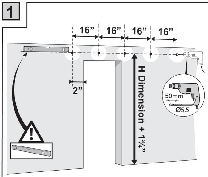
Find the centerline of the track. Using a level, mark a horizontal line twice the door width long. Mark the bracket screw locations into the wall blocking. Attach the wall portion of the brackets as shown.
