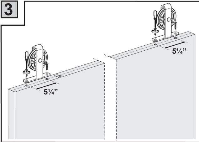
Drill holes in the top of the door 5-1/4" from the edge as pictured to accommodate the door rollers. The bottom of the door should be routed at this time in order to accept the floor guide.
