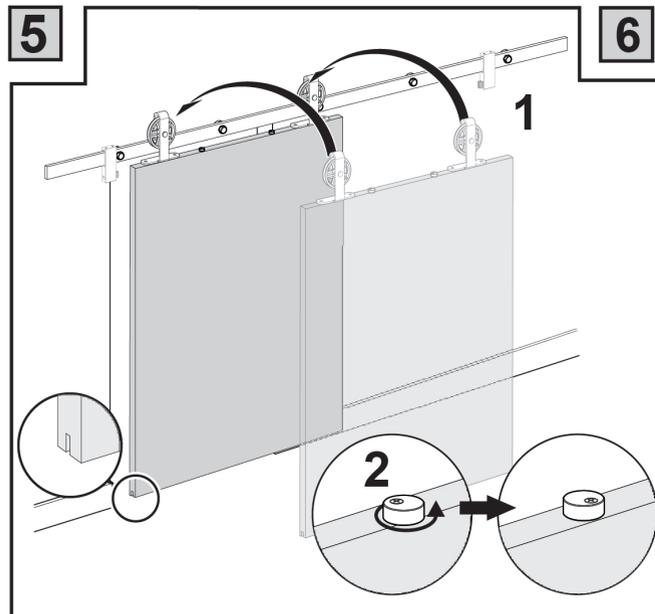
Attach the door to the rails making sure that the anti-jump disks are engaged to avoid a serious accident.
