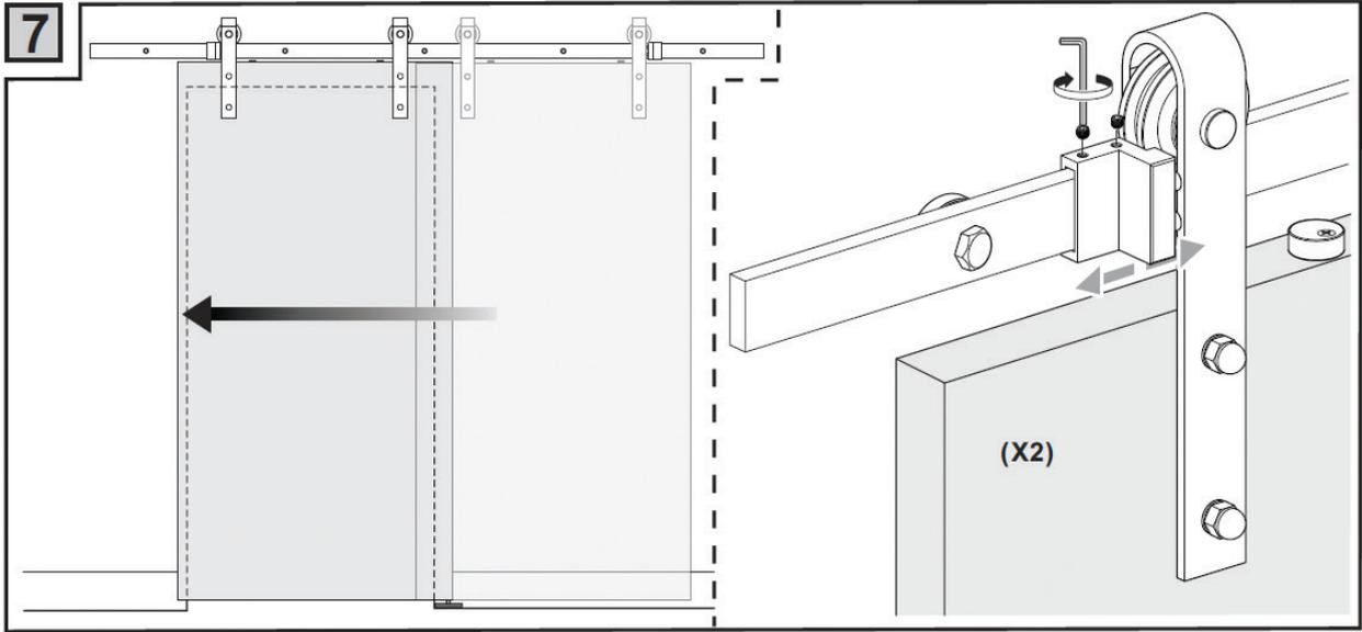
Adjust the door stops accordingly using the provided 2.5mm Allen key.
