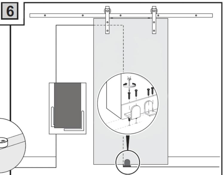
Plumb the door and mark the positions of the floor guides. Mount the floor guides to the floor.
