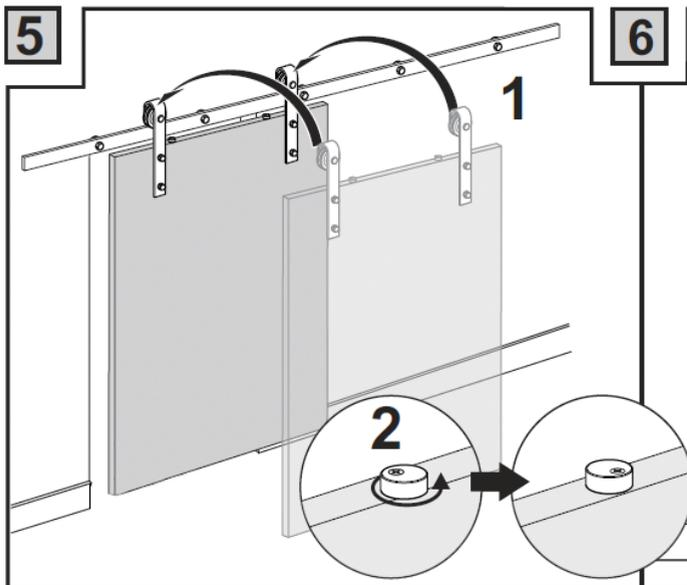
Attach the doors to the rails making sure that the anti-jump disks are engaged to avoid a serious accident.
